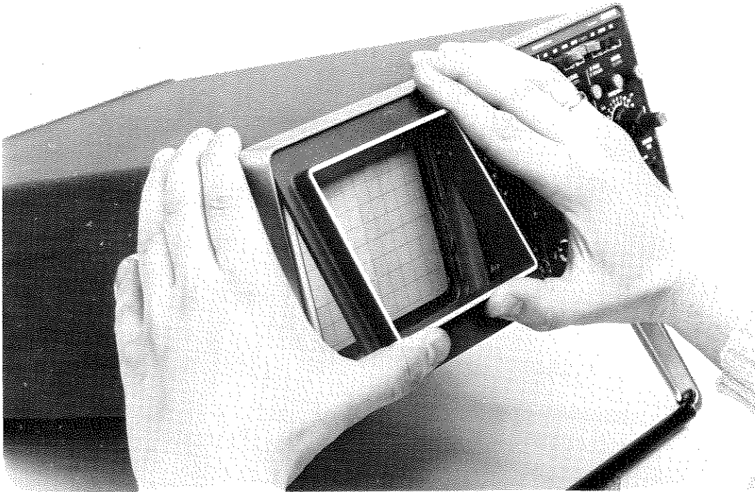
Fig. 2.9. Removing the bezel and the contrast plate
